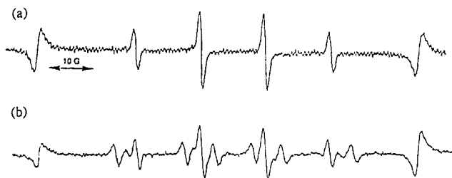
Figure 1. ESR spectrum of the hydroxyl radical spin adduct of DMPO produced during photoirradiation of hydroperoxide 7 . (a) The sample solution containing 1 \mu\text{L} of hydroperoxide 7 (10 mM) in acetonitrile, 5 \mu\text{L} of DMPO (29.2 mM), 10 \mu\text{L} of sodium cacodylate (20 mM), and 84 \mu\text{L} of water was irradiated with transilluminator (302 nm) at ambient temperature for 10 min. An aliquot (5 \mu\text{L} ) of the solution was taken up in a capillary, and the ESR was measured at room temperature. The magnetic fields were calculated by the splitting of \text{Mn}^{2+} in \text{MnO} ( \Delta H_{3-4} = 86.9 G) (signals at both ends). The 1:2:2:1 pattern of four lines can be interpreted in terms of equivalent hyperfine splitting constants ( a_{\text{N}} = a_{\text{H}} = 14.8 G, g = 2.0058 ) due to both the nitroxide nitrogen and the \beta -hydrogen. 14 (b) Addition of ethanol (2.5 mM), a hydroxyl radical scavenger, to the reaction system described above collapsed the signals of the DMPO-OH adduct, resulting in the production of signals due to \text{CH}_3\text{CHOH} . Similar ESR spectra were obtained in the photoirradiation of 2 and 9 .
